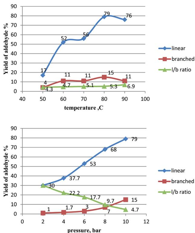
Fig. 2 Graphs depicting the influence of 1 : 1 CO–H<sub>2</sub> pressure and temperature on the selectivity of 1-hexene hydroformylation catalyzed by Rh/PAA + PPh<sub>3</sub>; [PPh<sub>3</sub>]/[Rh] = 13, [1-hexene]/[Rh] = 800.
