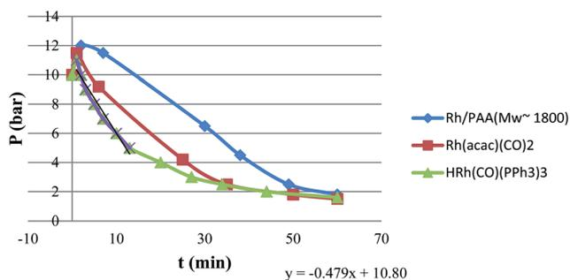
Fig. 3 Changes of H<sub>2</sub>/CO pressure vs. time during hydroformylation of 1-hexene catalyzed by Rh/PAA, Rh(acac)(CO)<sub>2</sub> and HRh(CO)(PPh<sub>3</sub>)<sub>3</sub> in the presence of PPh<sub>3</sub> ([PPh<sub>3</sub>]/[Rh] = 13) in water. [1-Hexene]/[Rh] = 800, *T* = 80 °C, H<sub>2</sub>-CO (1 : 1) = 10 bar. Linear approximation used for determination of TOF was shown for reaction with HRh(CO)(PPh<sub>3</sub>)<sub>3</sub>.
