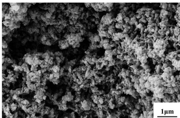
Fig. 3 SEM images of granular PANI powder morphology. Synthetic conditions: [aniline] = 0.5 M, [aniline]-[APS] = 2 : 1, [H<sub>3</sub>PO<sub>4</sub>] = 1 M.
