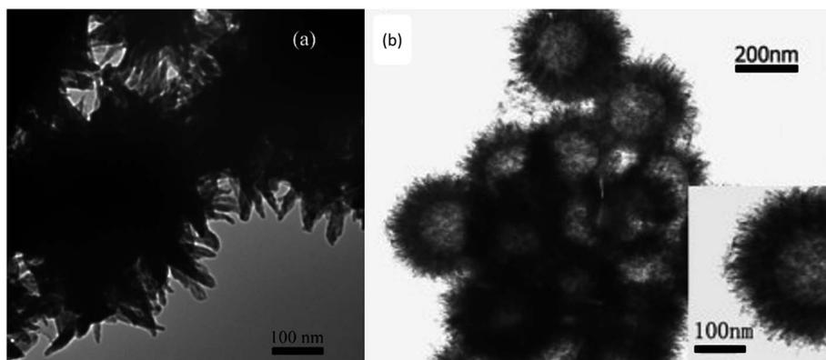
Fig. 7 TEM images of urchin-like (a) PANI nanorods prepared through the chemical polymerization of corresponding monomer complex ( $\beta$ -CD and aniline are in equal moles).<sup>81</sup> (b) PANI hollow spheres obtained by dispersing hollow spheres preloaded with anilinium salt solution into ferric chloride solution.<sup>82</sup>
