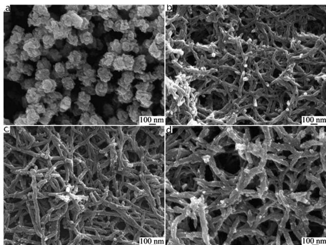
Fig. 4 SEM images of polyaniline nanofibers synthesized using different concentrations of HCl. (a) 0.01 M; (b) 0.2 M; (c) 0.5 M; (d) 1 M. Synthetic conditions: [aniline] = 0.05 M, [aniline]–[APS] = 4 : 1, [APS]–[Fe<sup>2+</sup>] = 3 : 2, and 6 h.<sup>68</sup>
