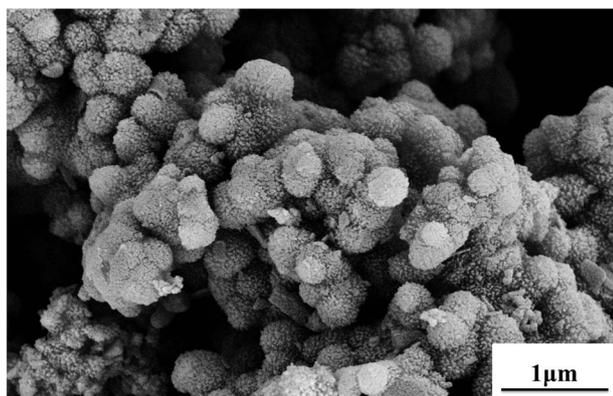
Fig. 6 SEM images of PANI nanosphere prepared in phosphoric acid. Synthetic conditions: [aniline] = 0.2 M, [aniline]–[APS] = 4 : 5, [H<sub>3</sub>PO<sub>4</sub>] = 1 M.
