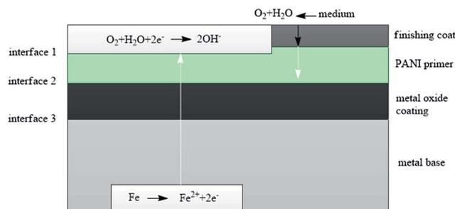
Fig. 11 Barrier protection mechanism of PANI.<sup>136</sup>
