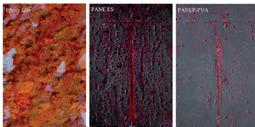
Fig. 8 Photograph of pure epoxy-coated panel, 2.5 wt% PANI ES-coated panel, and 2.5 wt% PANI/P-PVA-coated panel after 30 days of exposure to salt spray test.<sup>104</sup>
