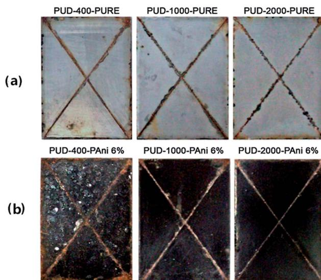
Fig. 9 Photographs showing MS panels coated with (a) pure and (b) blended polymers after exposing to salt spray test (300 h).<sup>108</sup>
