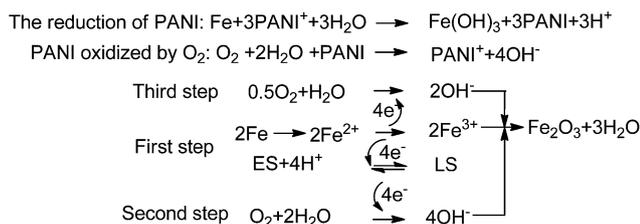
Scheme 3 Description of the catalytic passivation of iron by PANI.<sup>127</sup>
