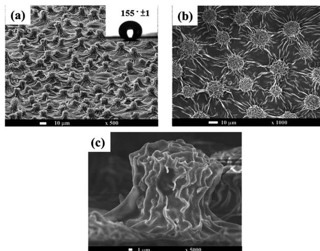
Fig. 10 SEM images of (a) *Xanthosoma sagittifolium* leaf-like superhydrophobic polymeric surface. Inset shows the contact angle of polymeric surface. (b) Top view of polymeric surface. (c) Cross-sectional view of polymeric surface.<sup>123</sup>
