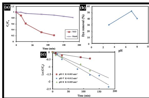
Fig. 8 (a) Variation in RB concentration with time (NiO dose ( $W$ ) =  $1 \text{ g L}^{-1}$ ,  $[\text{RB}] = 10 \text{ mg L}^{-1}$ ,  $\text{pH} = 7$ ), (b) pH effect on the removal of RB dye (NiO dose ( $W$ ) =  $1 \text{ g L}^{-1}$ ,  $[\text{RB}] = 10 \text{ mg L}^{-1}$ ,  $T = 20 \text{ }^\circ\text{C}$ ,  $t = 12 \text{ h}$ ), (c) effect of the initial pH on the photocatalytic degradation of RB dye (NiO dose ( $W$ ) =  $1 \text{ g L}^{-1}$ ,  $[\text{RB}] = 10 \text{ mg L}^{-1}$ ).
