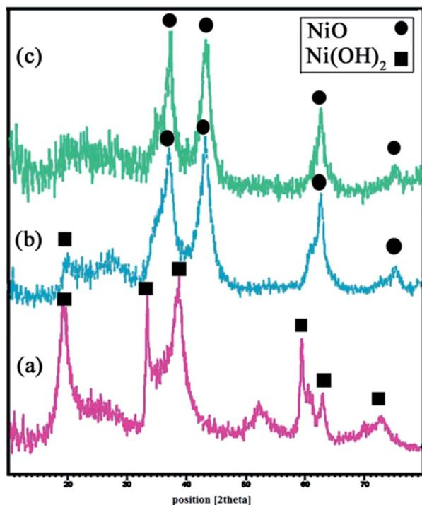
Fig. 3 XRD patterns of (a)  $\beta$ -Ni(OH)<sub>2</sub>, (b and c) 6 hours calcined  $\beta$ -Ni(OH)<sub>2</sub> at 700 °C and 750 °C, respectively.
