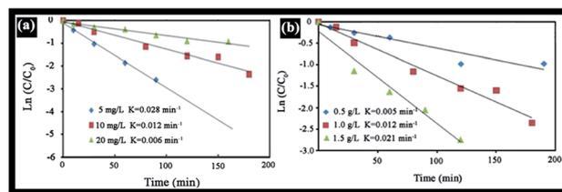
Fig. 10 (a) Effect of dye concentration on the photocatalytic degradation of RB dye (NiO dose (W) = 1 g L<sup>-1</sup>, pH = 7), (b) effect of photocatalyst concentration on the photocatalytic degradation of RB dye ([RB] = 10 mg L<sup>-1</sup>, pH = 7).
