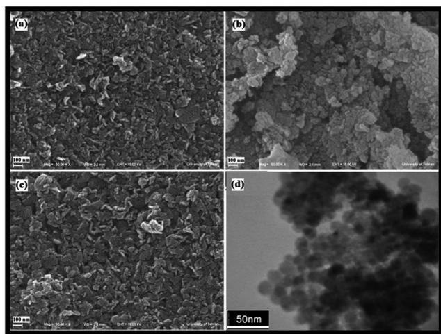
Fig. 4 FESEM images of (a) Ni(OH)<sub>2</sub> and Ni(OH)<sub>2</sub> calcined at (b) 700 °C and (c) 750 °C, and (d) TEM image of Ni(OH)<sub>2</sub> calcined at 750 °C.
