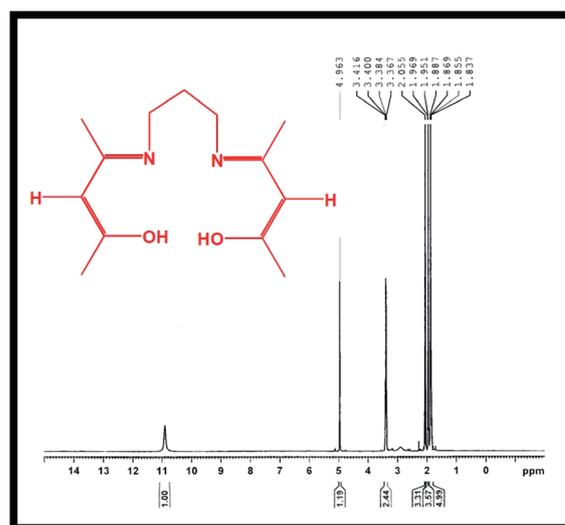
Fig. 2 <sup>1</sup>H-NMR of the H<sub>2</sub>(pnAA<sub>2</sub>) Schiff-base.
