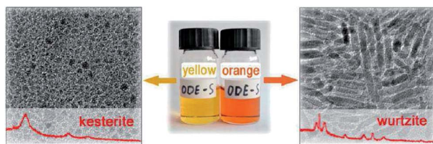
Fig. 27 CZTS NCs with kesterite and wurtzite structures were synthesised from metal acetate salts with either yellow or orange colour ODE-S as the sulfur precursor (reproduced with permission from ref. 171, copyright 2013, American Chemical Society).
