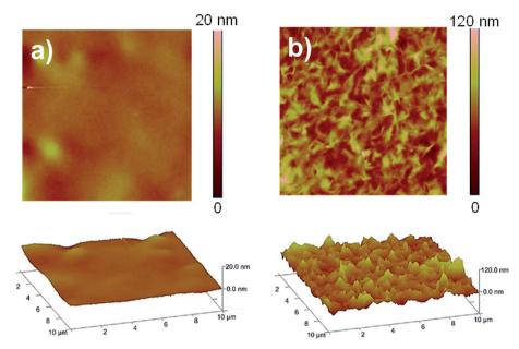
Fig. 8 Influence of the clay loading on the surface roughness of biopolymer coatings. AFM height (upper) and 3D (lower) images ( $10 \times 10 \ \mu m^2$ ) of pure pullulan coating (a) and pullulan/Na<sup>+</sup>-MMT nanocomposite coating (b) (filler volume fraction  $\varphi = 0.12$ ) (reproduced with permission from American Chemical Society<sup>19</sup>).
