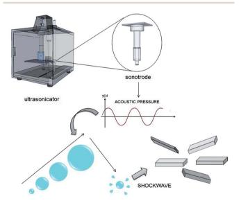
Schematic illustration of the ultrasonication method based on the acoustic cavitation. The sonotrode of an ultrasonicator generates high intensity ultrasound waves of alternating expansive and compressive cycles. This causes the formation, growth, and collapse of bubbles, which in turn yields intense shockwaves that promote interparticle collisions and, eventually, the exfoliation of the layered filler.
