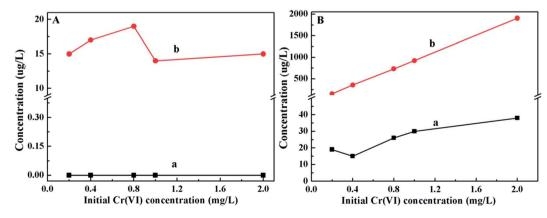
Fig. 6  $Cr(v_1)$  (a) and total Cr (b) concentrations in the solution (A) and PANI/CFs (B) after adsorption with initial  $Cr(v_1)$  concentrations ranging from 0.2 to 2.0 mg  $L^{-1}$ .
