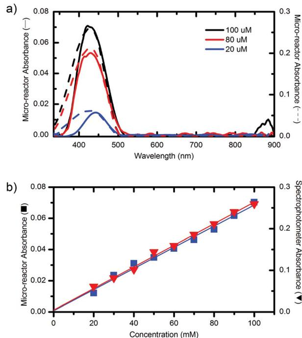
**Fig. 2** (a) Absorbance spectra collected with the microscope-coupled spectrophotometer from the microreactor (—), and with the bench spectrophotometer (---). (b) Absorbance of tartrazine solution measured with the microscope-coupled spectrophotometer (■), and with the bench spectrophotometer (▼) at a wavelength of 425 nm.
