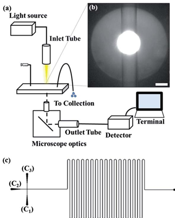
**Fig. 1** (a) Schematic layout of the experimental setup, (b) focused light spot on the microfluidic reactor channel (scale bar: 200  $\mu\text{m}$ ), and (c) the microfluidic reactor layout where  $C_1$ ,  $C_2$  and  $C_3$  are three channel inlets.
