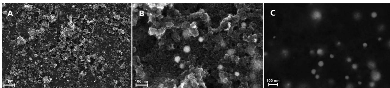
Fig. 5 SEM micrographs of the graphite-Ag-nanocomposite film: (A) at low magnification showing overall film morphology (the bright spots are Ag-NPs); (B) at higher magnification; (C) is a BS SEM micrograph of (B) displaying the morphology of the Ag-NPs (some of them are beneath the surface, hence the diffuse contrast).
