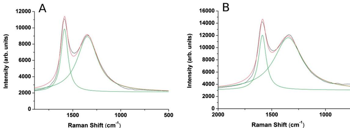
Fig. 2 The Raman scattering spectra of the nanographite films (A) plain graphite film; (B) the graphite–Ag nanocomposite film. The broad peak centred at  $1347\text{ cm}^{-1}$  is the D band, the narrower centred at  $1586\text{ cm}^{-1}$  is the G band.
