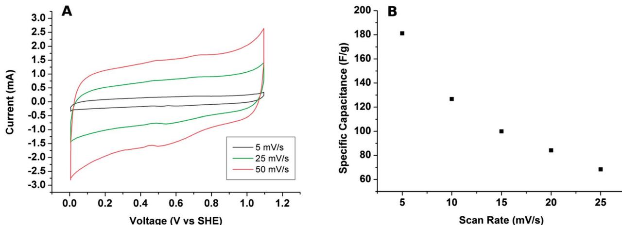
Fig. 7 (A) Current vs. voltage (CV) curves of the graphite films in a 0.5 M  $\text{H}_2\text{SO}_4$  electrolyte for 3 different voltage scans; (B) plot of the specific capacitance as a function of the scan rate.
