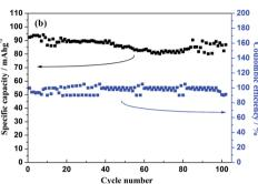
Fig. 12 (a) Initial charge/discharge profiles of  $Na_3V_2(PO_4)_2F_3$  hybridion battery at 0.091 C. (b) The cycling performances of  $Na_3V_2(PO_4)_2F_3$  hybridion battery at 0.91 C.
