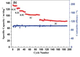
Fig. 11 (a) Initial charge/discharge profiles of  $Na_3V_2(PO_4)_2F_3$  hybridion batteries at different current densities. (b) The C-rate and cycling performances of  $Na_3V_2(PO_4)_2F_3$  hybridion battery.
