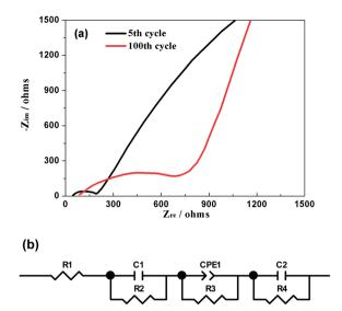
Fig. 13 (a) Nyquist plots of the hybrid-ion battery charged to 3.2 V vs. Li<sup>+</sup>/Li for the 5th and 100th cycle. (b) The equivalent circuit model.
