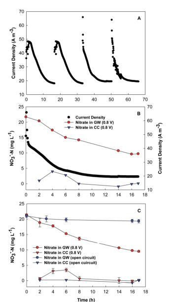
Fig. 2 The BES performance: (A) current generation; (B) the correlation between nitrate concentration and current generation; and (C) the nitrate concentrations under the open - and the closed - circuit conditions. GW: groundwater; CC: concentrating chamber.
