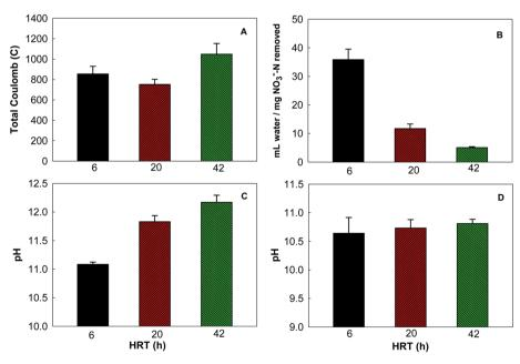
Fig. 3 The results of varying the flow rate (or HRT as shown by the x-axis) of the DI water supply to the concentrating chamber: (A) total Coulomb production; (B) the water consumption per mg nitrate nitrogen removed; (C) the pH of the water in the concentrating chamber; and (D) the pH of the synthetic groundwater.
