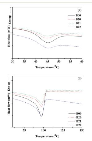
Fig. 4 DSC thermograms for B00, B20, B21 and B22 compositions (a) order–disorder transition temperatures observed during first heating cycle (b) PEMA melting peaks from the second heating cycle.
