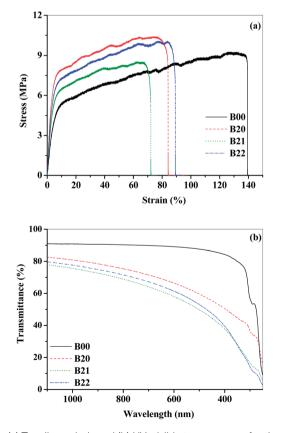
Fig. 5 (a) Tensile analysis and (b) UV-visible transparency for the neat, blend and composite films.
