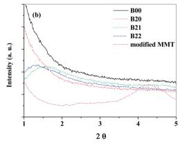
Fig. 2 (a) FTIR spectra and (b) XRD peaks referring to gallery spacing for the neat (B00), blend (B20) and composite (B21, B22).
