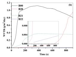
Fig. 6 Values for the neat, blend and composite films determined (a) OTR from calcium degradation test (b) WVTR from CRDS based permeability setup.
