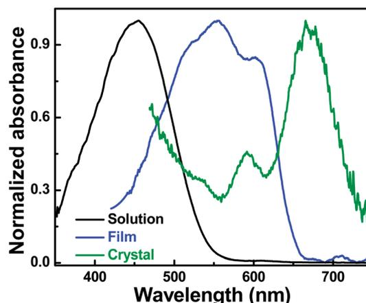
Fig. 1 Normalized UV-Vis absorption spectra of P3HT: 3-hexylthiophene solution (0.2 mg ml<sup>−1</sup>) at 50 °C (black), thin film of a thickness of  $\sim 65$  nm spin-cast from a homogeneous solution in 3-hexylthiophene (blue) and a single crystal of a thickness of  $\sim 59$  nm (olive) spin cast from a 3-hexylthiophene dispersion.
