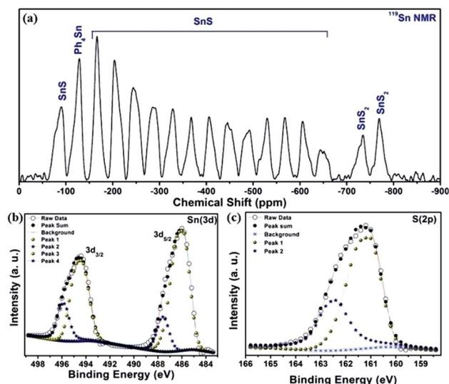
Fig. 2 (a) <sup>119</sup>Sn solid-state CP-MASS NMR spectrum of SnS NRs, (b) X-ray photoelectron spectra (XPS) for Sn (3d) and (c) for S (2p) of SnS NRs.
