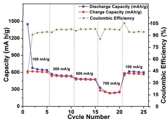
Fig. 8 Power plot with coulombic efficiency for SnS nanorods-CMC electrode in a potential window of 0.01–1.2 V vs. Li/Li<sup>+</sup> at 20 °C.
