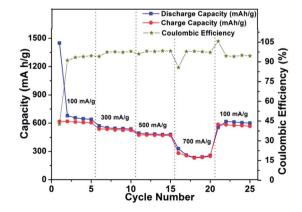
Fig. 8 Power plot with coulombic efficiency for SnS nanorods–CMC electrode in a potential window of  $0.01-1.2~V~vs.~Li/Li^+$  at  $20~^{\circ}C.$
