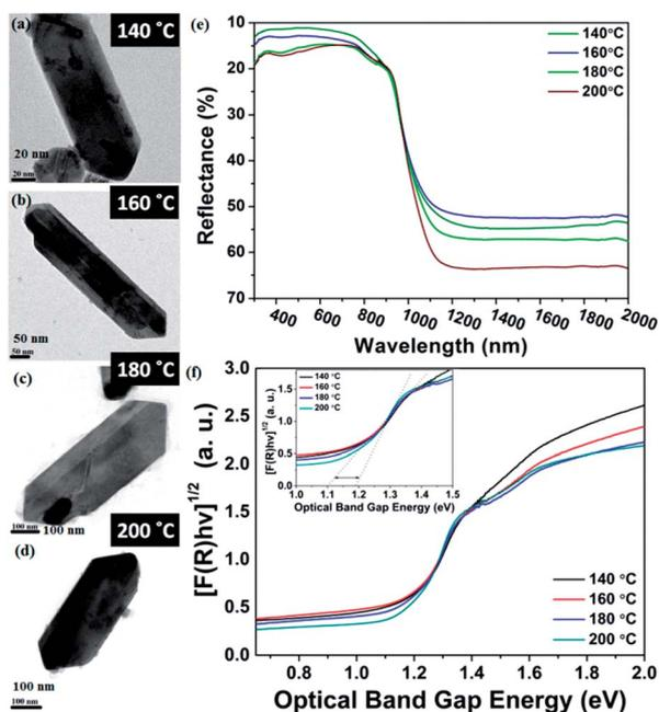
Fig. 6 Optical property and FEG-TEM images of SnS NRs synthesized at (a) 140 °C, (b) 160 °C, (c) 180 °C and (d) 200 °C. (e) Reflectance vs. wavelength plot. (f) Band gap measurement with help of  $(\alpha h\nu)^{1/2}$  vs.  $E_g$  plot (Tauc's plot)
