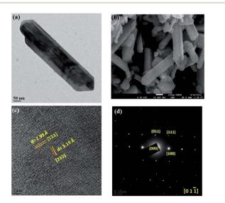
Fig. 3 Electron microscopy patterns of SnS NRs synthesized at  $160\,^{\circ}$ C: (a) FEG-TEM image of single SnS NRs, (b) FEG-SEM image, (c) high resolution lattice fringe and (d) SAED pattern from zonal axis [0 1 -1].
