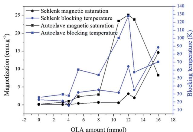
Fig. 3 Saturation magnetisation and blocking temperature of samples synthesised on a Schlenk line (from left to right, samples 7–15) and in an autoclave (from left to right, sample 17–25). The data were extracted from the hysteresis loops and ZFC–FC curves in Fig. S8.†
