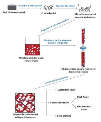
Fig. 4 Schematic illustration showing how nano/submicron particulates can be prepared, from starting bulk materials to study the toxicity of biomaterial eluates.<sup>176</sup>
