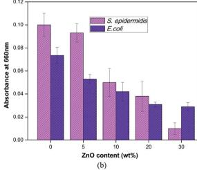
Fig. 7 (a) MTT assay results showing the viable SaOS2 osteoblast-like cells and L929 fibloblasts cells on monolithic HA and HA with varying ZnO content after 7 days of culture.<sup>67</sup> (b) Mean optical density data after 4 hours of incubation with *S. epidermidis* and *E. coli* on pure HA and HA with increase in ZnO content.<sup>157,162</sup>
