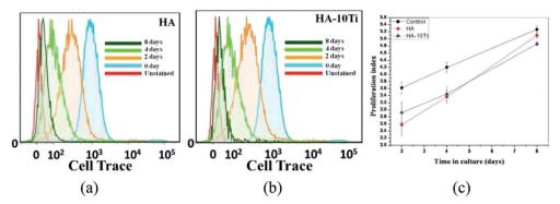
Fig. 6 Representation of flow cytometry data, showing the proliferation of hFOB 1.19 cells incubated for various time periods. Graphical representations of flow cytometry data, showing the cell proliferation viz. dye reduction for (a) HA and (b) HA10Ti and proliferation index (c).<sup>152</sup>
