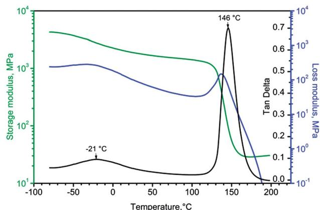
Fig. 11 DMA curves for the DGEBA/DETA cured system.
