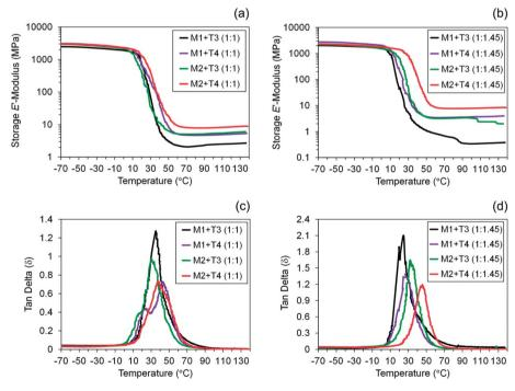
Fig. 9 Influence of the type of thiol–ene formulation (combination and stoichiometry) on the thermo-viscoelastic properties of the final cured films. Plots (a) and (b) storage modulus *versus* temperature; and, plots (c) and (d) tan  $\delta$  (E''/E') *versus* temperature.
