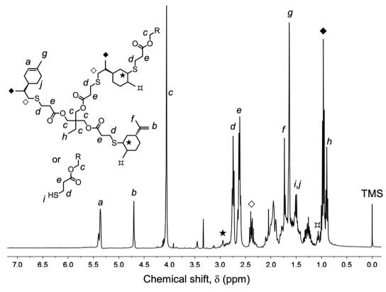
Fig. 4 Representative <sup>1</sup>H-NMR (400 MHz, CDCl<sub>3</sub>) spectrum of resin 1 (TE-C1) with principal signal assignments resulting from photoinduced thiol-ene coupling between compounds 1 and 2 reacted at an initial stoichiometry of 1: 0.5. The synthesis reaction was conducted for a period of 6 hours at room temperature in EtOAc solution. Integration value of the ethyl ester proton signal (c) was used as a reference peak for the calculation of double-bond conversion.
