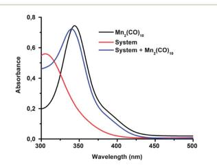
Fig. 1 UV-Vis spectra of Mn<sub>2</sub>(CO)<sub>10</sub>, reaction mixture and both of them in methanol. The concentration of all components was  $2.3\times10^{-3}$  M.
