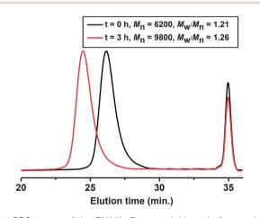
Fig. 7 GPC traces of the PMMA–Br macroinitiator before and after chain extension via visible light-induced ATRP using Mn<sub>2</sub>(CO)<sub>10</sub>. Experimental conditions: [MMA]<sub>0</sub>/[PMMA–Br]<sub>0</sub>/[Cu<sup>II</sup>Br<sub>2</sub>]<sub>0</sub>/[PMDETA]<sub>0</sub>/[Mn<sub>2</sub>(CO)<sub>10</sub>]<sub>0</sub> = 200/1/0.01/0.01/0.05 ratio.
