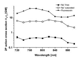
Fig. 2 2P fluorescence excitation action cross-sections  $\Phi_F \sigma_2$  of Na<sup>+</sup>free and  $Na^+$ -saturated ANG-2 buffer solutions (N = 6 for each form). For the reference fluorescein (in NaOH, pH 11) literature data were used; <sup>18</sup> 1 GM =  $10^{-50}$  cm<sup>4</sup> s per photon;  $\Phi_{\rm F}\sigma_2$  is the product of 2P absorption cross-section  $\sigma_2$  and fluorescence quantum yield  $\Phi_{\rm F}$ .
