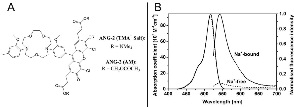
Fig. 1 (A) Chemical structure of ANG-2.<sup>20</sup> (B) Absorption and normalised fluorescence spectra of Na<sup>+</sup>-bound (solid lines) and Na<sup>+</sup>-free (dashed lines) form of ANG-2 with excitation wavelength  $\lambda_{\text{ex}} = 517 \text{ nm}$  and  $c_{\text{dye}} = 1.3 \mu\text{M}$ .
