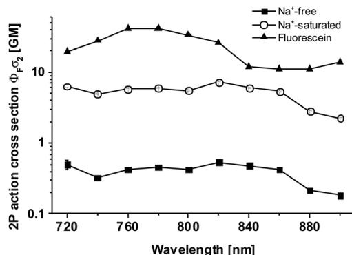
Fig. 2 2P fluorescence excitation action cross-sections  $\Phi_{\text{F}\sigma_2}$  of Na<sup>+</sup>-free and Na<sup>+</sup>-saturated ANG-2 buffer solutions ( $N = 6$  for each form). For the reference fluorescein (in NaOH, pH 11) literature data were used;<sup>18</sup>  $1 \text{ GM} = 10^{-50} \text{ cm}^4 \text{ s per photon}$ ;  $\Phi_{\text{F}\sigma_2}$  is the product of 2P absorption cross-section  $\sigma_2$  and fluorescence quantum yield  $\Phi_{\text{F}}$ .
