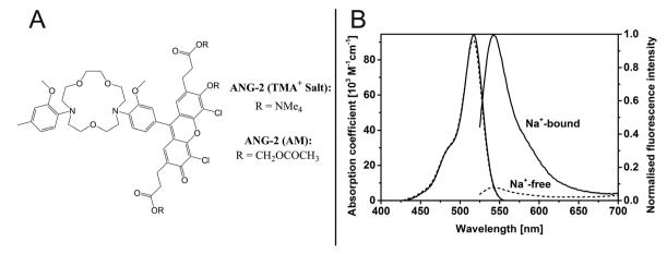
Fig. 1 (A) Chemical structure of ANG-2.<sup>20</sup> (B) Absorption and normalised fluorescence spectra of Na<sup>+</sup>-bound (solid lines) and Na<sup>+</sup>-free (dashed lines) form of ANG-2 with excitation wavelength  $\lambda_{\rm ex}$  = 517 nm and  $c_{\rm dye}$  = 1.3  $\mu$ M.
