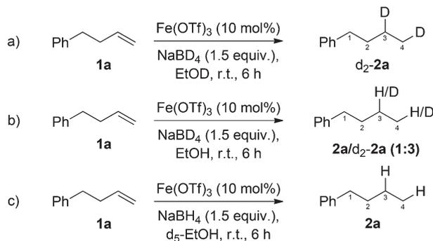
**Scheme 3** Deuterium labelling studies for the investigation of the mechanism of iron-catalysed, NaBH<sub>4</sub> mediated, alkene reduction.
