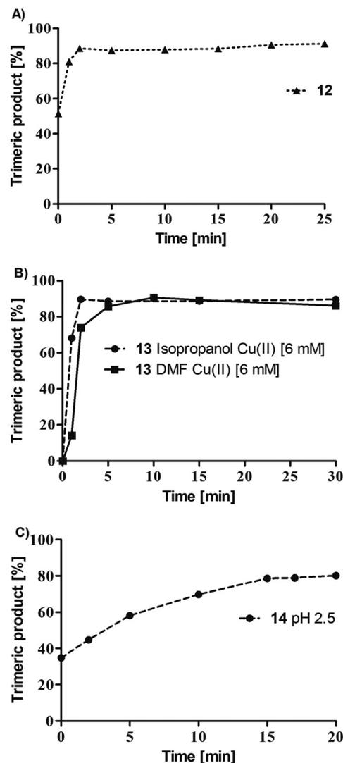
Fig. 2 Kinetics of ligation reactions: (A) thioether ligation (generation of **12**), (B) 1,3-dipolar cycloaddition (generation of **13**), (C) oxime ligation (generation of **14**). Monomeric peptides were used at 3 mM and scaffolds at 1 mM, resulting in a concentration of 1 mM for the generated trivalent peptides.
