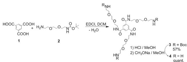
**Scheme 1** Synthesis of the amino-functionalized trimesic acid scaffold **4**.
