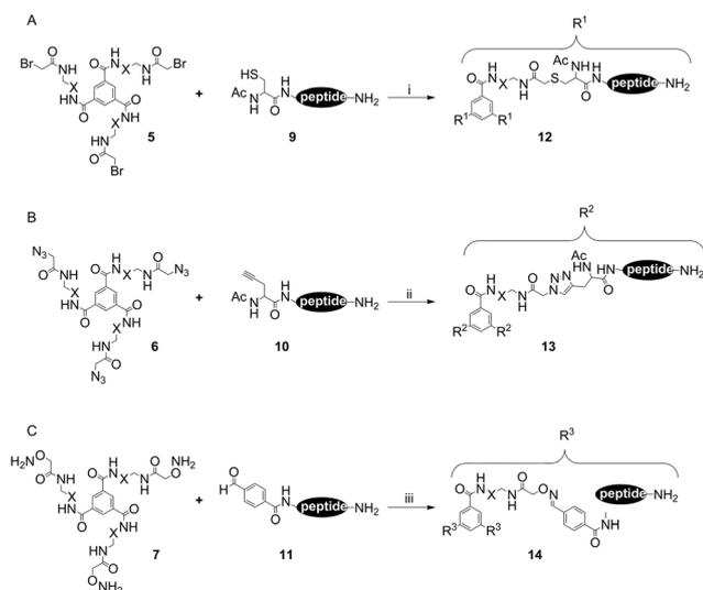
Scheme 3 Ligation reactions. (A) Thioether ligation; (B) 1,3-dipolar cycloaddition; (C) oxime ligation. (i) Carbonate buffer pH 9.6; (ii) 6 M CuSO<sub>4</sub>, 18 M sodium ascorbate; (iii) citrate buffer pH 2.5. X: -(CH<sub>2</sub>)<sub>2</sub>-O-(CH<sub>2</sub>)<sub>2</sub>-O-(CH<sub>2</sub>)<sub>2</sub>-; peptide: Ahx-AKIYRP.
