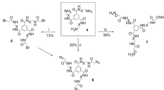
**Scheme 2** Functionalization of the amino scaffold **4** for different ligation reactions. (i) Bromoacetic acid/DIC; (ii) azidoacetic acid/EDCI; (iii) (a) AOA/EDCI, (b) TFA/DCM; X:  $-(CH_2)_2-O-(CH_2)_2-O-(CH_2)_2-$ .
