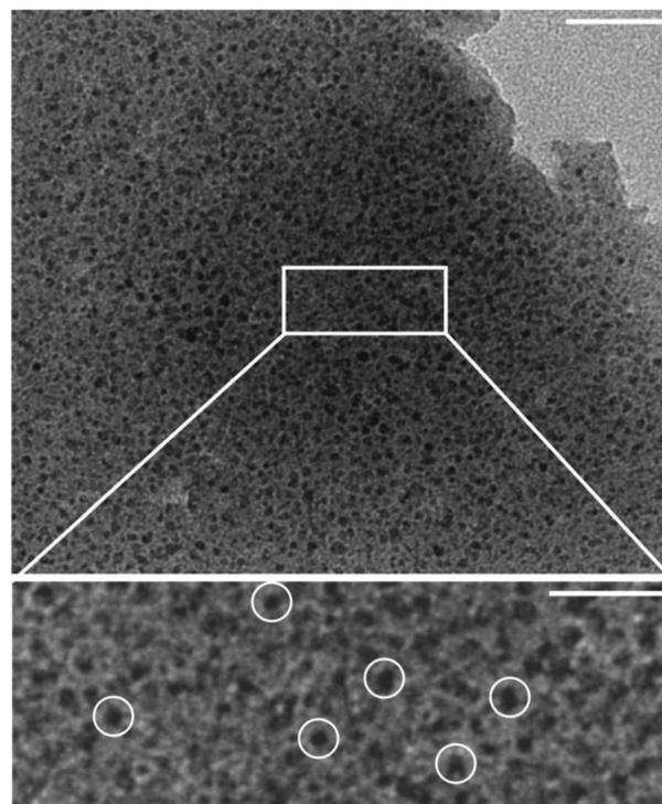
**Fig. 5** TEM images of  $\text{BaCO}_3$  nanoclusters (black spots) that are distributed throughout a matrix of lower electron contrast, presumably consisting of amorphous silica. These structures were isolated immediately after the maximum in free  $\text{Ba}^{2+}$  concentration had been reached in titrations at pH 10.5 and 600 ppm  $\text{SiO}_2$ . Scale bars are 40 nm (overview) and 20 nm (zoom).
