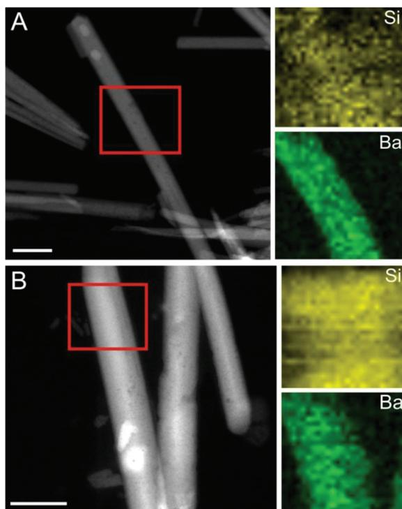
**Fig. 4** STEM images and the corresponding Si and Ba elemental maps for  $\text{BaCO}_3$  nanorods formed during titration of  $\text{BaCl}_2$  into carbonate buffer at pH 10, containing (A) 300 and (B) 600 ppm silica. The red rectangle marks the region analysed by EDX. The data show that increased counts of silicon are detected around the carbonate particles. Scale bars are 100 nm.
