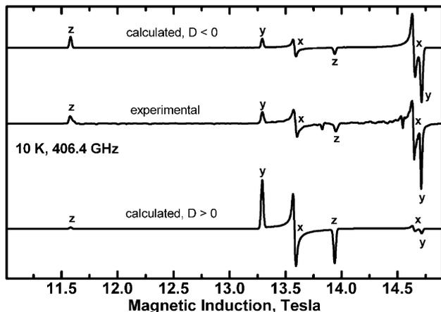
Fig. 14 Determination of the sign of the zero-field splitting parameters from the high-frequency EPR spectra recorded at 10 K with  $\nu = 406.4$  GHz. The sign of  $D$  and  $E$  does not affect the positions of the resonance lines, but it does affect the intensity pattern at low temperatures and high frequencies. The spin Hamiltonian parameters at 10 K are:  $g_x = 2.056$ ,  $g_y = 2.045$ ,  $g_z = 2.320$ ,  $D = -1.042$   $\text{cm}^{-1}$ ,  $E = -0.0075$   $\text{cm}^{-1}$ .
