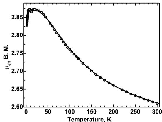
Fig. 10 The effective magnetic moment of **3** as a function of temperature. Dots: experimental, solid line – calculated with  $J = -100 \text{ cm}^{-1}$  (see the text).
