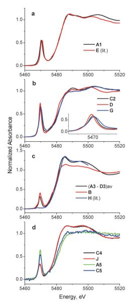
Fig. 3 Comparison of selected XANES spectra of the reaction products of A-D with those of model V(v), V(IV) and V(III) complexes (see also Fig. S1 and S2 in ESI;† designations correspond to those in Chart 1 and Table 1). All the data were collected at ~295 K in fluorescence detection mode for solid samples (freeze-dried reaction mixtures or mixtures of model complexes with BN; see Experimental section for details)
