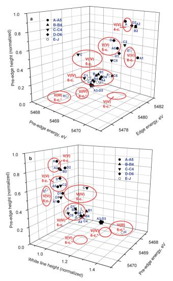
Fig. 2 Correlations of pre-edge and edge parameters in the XANES of the reaction mixtures (designations correspond to those in Table 1) and model complexes (Chart 1). The areas corresponding to various oxidation states and coordination numbers of V complexes (red ellipses) were drawn based on the XANES data for a library of twenty-three model V(v), V(iv) and V(iii) complexes (asterisks designate non-oxido complexes).<sup>22</sup>
