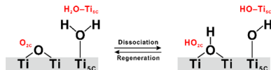
Fig. 4 Schematic diagram of H 2 O dissociation and regeneration on the TiO 2 surface.
