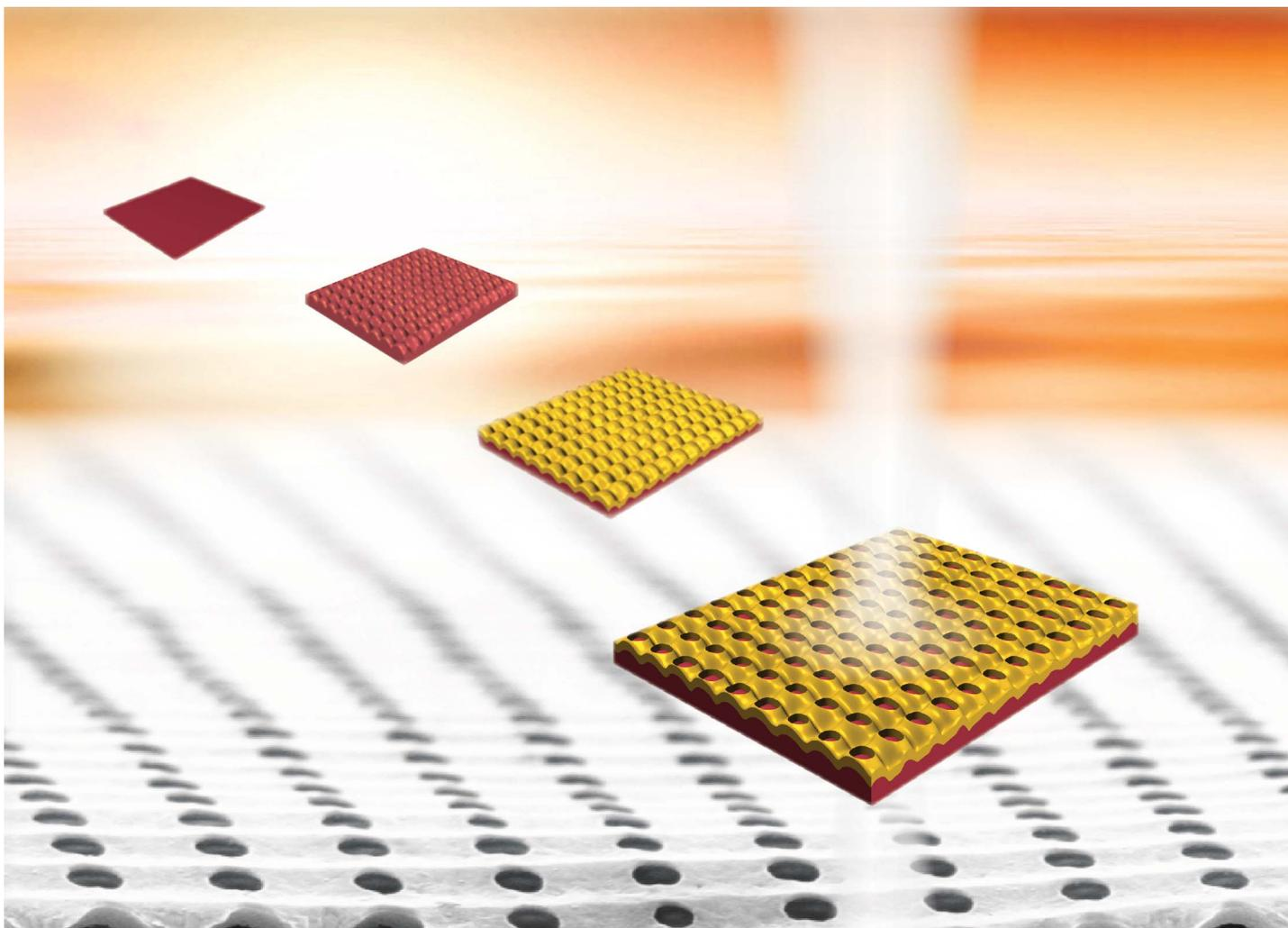
**An interdisciplinary team of scientists from Aalto University in Finland developed an efficient way to create large arrays of plasmonic structures with photo-moldable polymers.**
