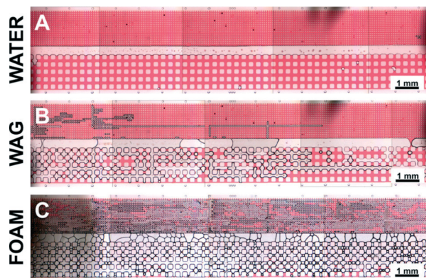
Fig. 3 Stacked-image comparisons of A) water flooding, B) water/air flooding without surfactant (WAG), and C) foam flooding at 4 min. Areas of red indicate unswept oil. The liquid flow rate and gas pressure were set to 0.05 \text{ mL h}^{-1} and 200 mbar, respectively.
