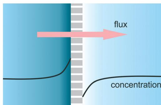
Fig. 3 Cartoon of a concentration polarization functional unit, based on selective transport through nanochannels, nanopores, gels, frits or membranes.
