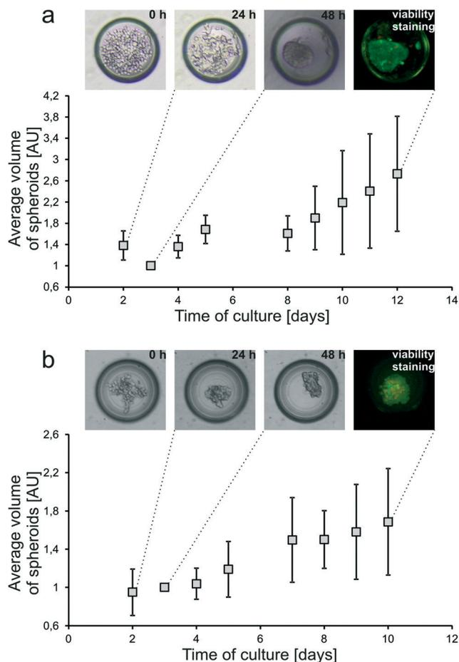
**Fig. 4** Growth of (a) HT-29 and (b) Hep-G2 spheroids in a microfluidic chip. Growth curves expressed in volumes of biomass normalized to 1 on the second day of culture (time of compact spheroid formation). Sequential micrographs present: (0 h) cells seeded to a microwell, (24 h) cell aggregation, (48 h) compact spheroid formation, and (viability staining) live/dead cell viability assay at the end-point of culture.
