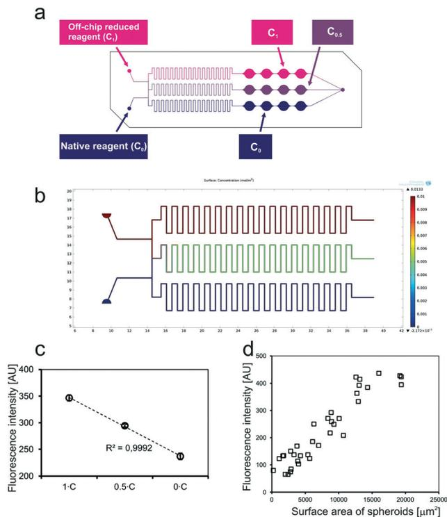
**Fig. 3** Proving the principle of measurements: (a) scheme of the experiment; (b) results of computational modelling of a CCG structure; (c) results of spectrofluorimetric measurements of the chip containing solutions as shown in scheme “a”. (d) Dependence of the fluorescence signal of one microchamber on the average size of spheroids in this chamber (on-chip culture).
