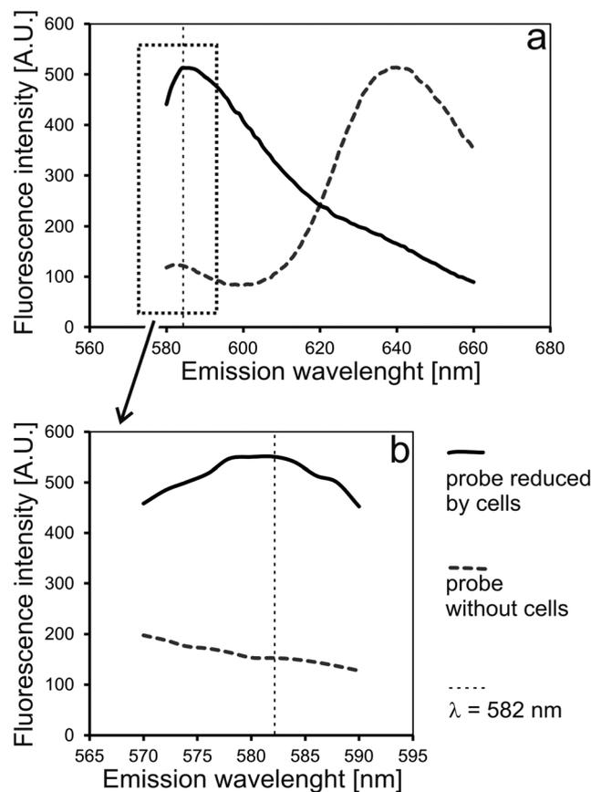
**Fig. 2** Comparison of emission spectra of alamarBlue reduced by cells (off-chip) and native form of alamarBlue in cell culture medium (without cells). Measurements performed: (a) in a standard 1 cm quartz cuvette and (b) on a microfluidic chip placed in a microplate reader. Excitation wavelength = 552 nm.
