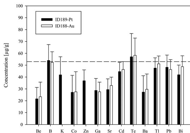
Fig. 4 Results of the analysis of synthetic fluid inclusions from experiment *ID188-Au* (white columns) and *ID189-Pt* (black columns). The dashed line represents the starting composition of the experimental fluid, which was identical for both experiments. Only B, K, Cd, Te, Tl, Pb and Bi (for *ID188-Au*) could be fully recovered in the inclusions. Error bars show 1SD of the mean values from all analyzed inclusions from the specific sample.
