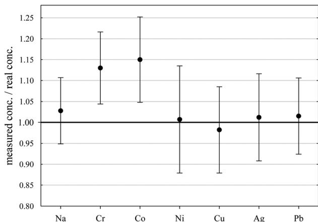
Fig. 3 Analysis of a self-prepared frozen standard solution against NIST610 glass. The real concentration of all elements is  $108\text{ }\mu\text{g g}^{-1}$ . Error bars show 1RSD values of 11 analyses.
