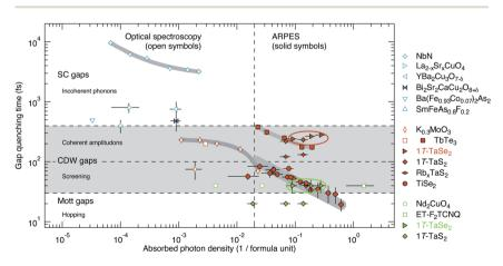
Fig. 6 Quenching times of electronic order parameters as a function of excitation density, as measured by time-resolved optical and photoemission spectroscopy for various superconductors, charge-density-wave systems, and Mott insulators. Data compiled from ref. 8–10, 17, 27 and 47–51. The results of this work are highlighted by ellipses.
