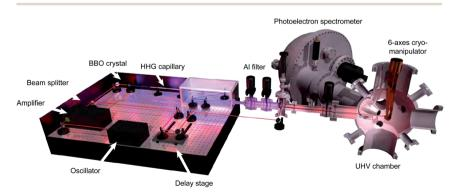
Fig. 2 Schematic illustration of the experimental setup for time-resolved high-harmonic-generation-based XUV-ARPES. Key components are labeled. For details, see text.
