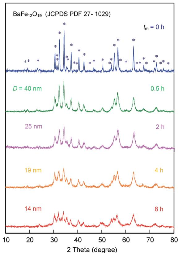
Fig. 4 The XRD patterns of BaFe<sub>12</sub>O<sub>19</sub> milled for various milling times. All diffraction peaks of bulk BaFe<sub>12</sub>O<sub>19</sub> (denoted by stars) can be indexed to the hexagonal magnetoplumbite structure with the space group *P6<sub>3</sub>/mmc*. The milling times (*t<sub>m</sub>*) and the corresponding average crystallite sizes (*D*) are shown in the figure.
