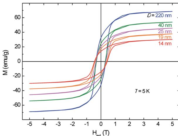
Fig. 8 Magnetization hysteresis loops for bulk and nanoscale mechanically treated  $\text{BaFe}_{12}\text{O}_{19}$ . Hysteresis loops were measured at 5 K after field cooling with  $H_{\text{ext}} = 5$  T. The average crystallite sizes of the  $\text{BaFe}_{12}\text{O}_{19}$  samples are shown in the figure.
