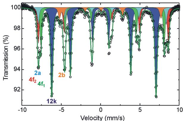
Fig. 2 The room temperature  $^{57}\text{Fe}$  Mössbauer spectrum of the standard  $\text{BaFe}_{12}\text{O}_{19}$  sample. The red, blue, cyan, green and orange colours denote the subspectra corresponding to the  $\text{Fe}^{3+}$  cations in the  $4f_2$ ,  $12k$ ,  $2a$ ,  $4f_1$ , and  $2b$  sublattices, respectively.
