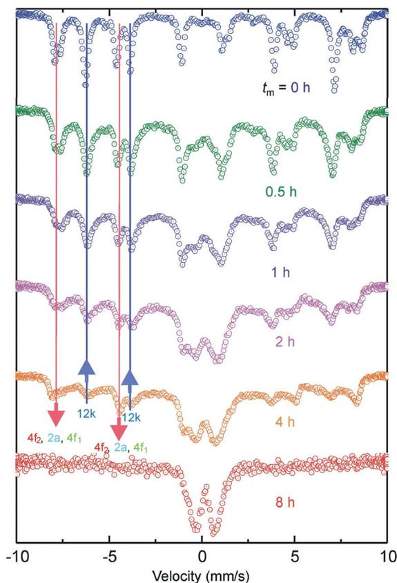
Fig. 5 The room temperature  $^{57}\text{Fe}$  Mössbauer spectra of  $\text{BaFe}_{12}\text{O}_{19}$  milled for various milling times (shown in the figure). The arrows emphasize the redistribution of the spectral intensities corresponding to the  $\text{Fe}^{3+}$  cations in the  $4f_2$ ,  $2a$ ,  $4f_1$  (red arrow) and  $12k$  (blue arrow) crystal sites of the ferrite.
