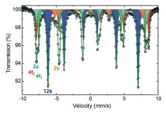
Fig. 2 The room temperature  $^{57}$ Fe Mössbauer spectrum of the standard BaFe $_{12}O_{19}$  sample. The red, blue, cyan, green and orange colours denote the subspectra corresponding to the Fe $^{3+}$  cations in the 4f2, 12k, 2a, 4f1, and 2b sublattices, respectively.
