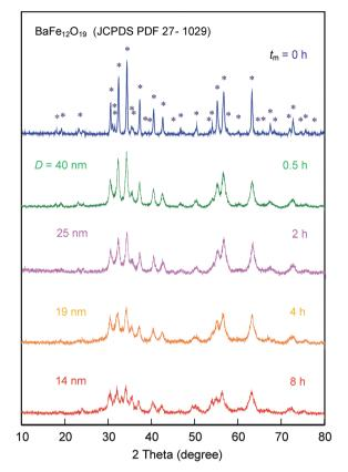
Fig. 4 The XRD patterns of BaFe $_{12}O_{19}$  milled for various milling times. All diffraction peaks of bulk BaFe $_{12}O_{19}$  (denoted by stars) can be indexed to the hexagonal magnetoplumbite structure with the space group  $P6_3/mmc$ . The milling times ( $t_m$ ) and the corresponding average crystallite sizes (D) are shown in the figure.
