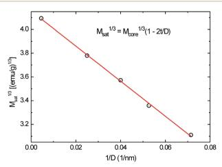
Fig. 9  $M_{\text{sat}}^{1/3}$  vs 1/D plot, where  $M_{\text{sat}}$  is the saturation magnetization and D is the diameter of the BaFe<sub>12</sub>O<sub>19</sub> nanoparticles.
