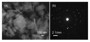
Fig. 1 (a) The electron microscopy image and (b) the corresponding SAED pattern illustrating the presence of hexagonal platelet crystals in the co-precipitated BaFe<sub>12</sub>O<sub>19</sub>.
