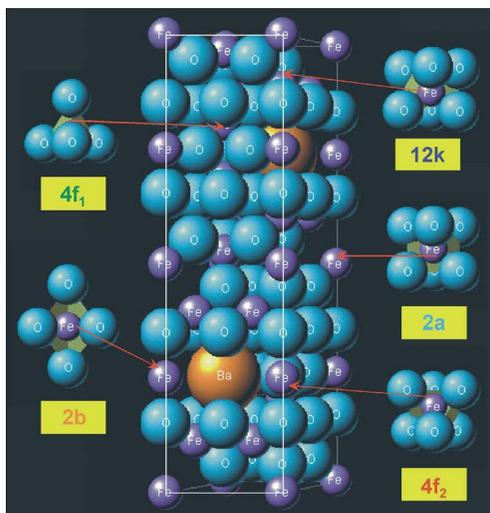
**Fig. 3** The crystal structure of the M-type hexaferrite.  $\text{Fe}^{3+}$  cations are distributed over the sites of octahedral ( $4f_2$ , 12k, 2a), tetrahedral ( $4f_1$ ) and trigonal bi-pyramidal (2b) coordination.
