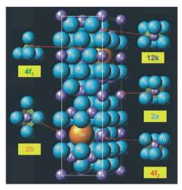
Fig. 3 The crystal structure of the M-type hexaferrite. Fe $^{3+}$  cations are distributed over the sites of octahedral (4f<sub>2</sub>, 12k, 2a), tetrahedral (4f<sub>1</sub>) and trigonal bi-pyramidal (2b) coordination.
