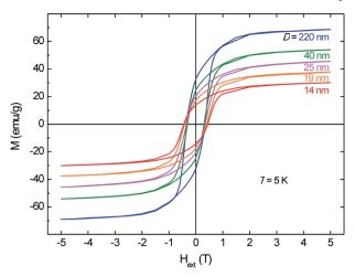
Fig. 8 Magnetization hysteresis loops for bulk and nanoscale mechanically treated  $BaFe_{12}O_{19}$ . Hysteresis loops were measured at 5 K after field cooling with  $H_{\rm ext}=5$  T. The average crystallite sizes of the  $BaFe_{12}O_{19}$  samples are shown in the figure.
