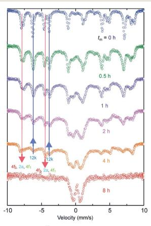
Fig. 5 The room temperature  $^{57}$ Fe Mössbauer spectra of BaFe $_{12}$ O $_{19}$  milled for various milling times (shown in the figure). The arrows emphasize the redistribution of the spectral intensities corresponding to the Fe $^{3+}$  cations in the 4f $_2$ , 2a, 4f $_1$  (red arrow) and 12k (blue arrow) crystal sites of the ferrite.
