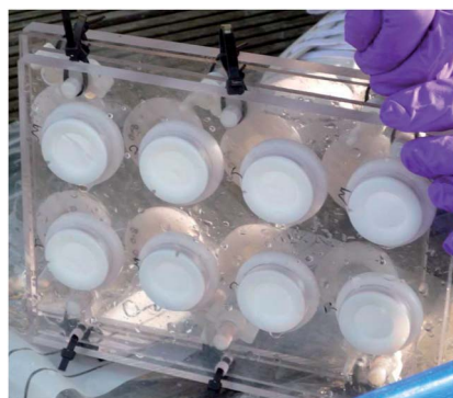
Fig. 2 Photograph of DGTs held in place by a Perspex plate. The plate held up to eight devices. If more samplers were deployed then two Perspex plates were fixed back to back. The plate was deployed in the rivers a vertical position.
