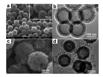
Fig. 5 (a) FESEM and (b) TEM images of HCS-PANI. (c) FESEM and (d) TEM images of GHCS-MnO $_2$ . Reproduced with permission from ref. 37 and 38. Copyright: 2010 American Chemical Society and 2012 The Royal Society of Chemistry.
