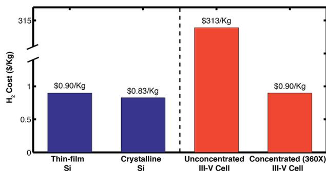
Fig. 7 Comparison of H<sub>2</sub> production costs from devices based on different PV technologies (unconcentrated Si cells in blue, and III-V cells in red). The cost shown for a concentrated cell, is the base H<sub>2</sub> cost and does not include the cost for the concentrator and tracking components.
