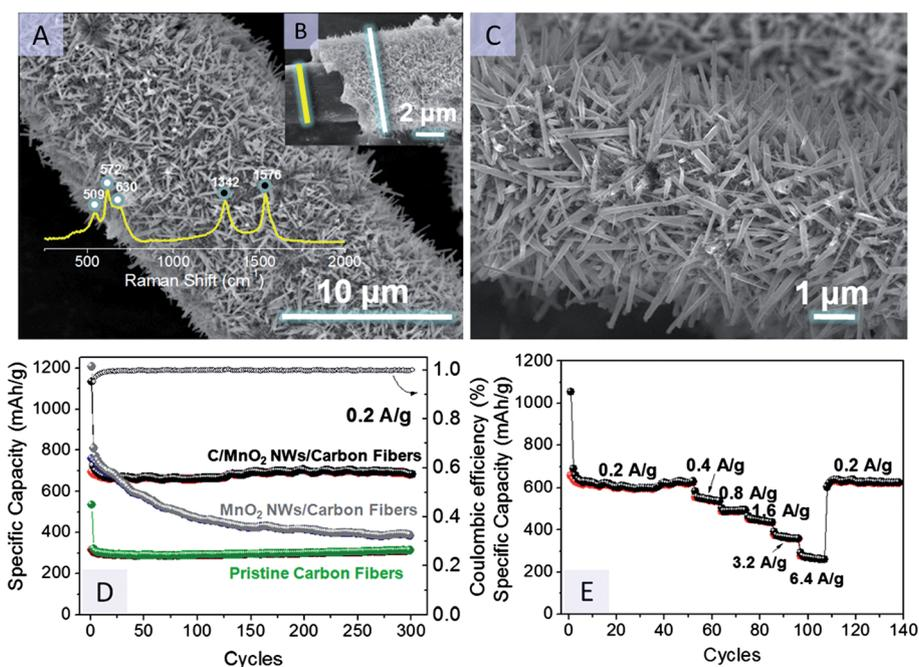
Fig. 5 (A–C) SEM observations toward the C/MnO<sub>2</sub> NWs/carbon fibers hybrid. The inset in (A) shows the Raman spectrum of this hybrid sample. (D) Cycling performance of C/MnO<sub>2</sub> NWs/carbon fibers, MnO<sub>2</sub> NWs/carbon fibers and the pristine carbon fibers performed at  $\sim 0.2$  A g<sup>-1</sup> for 300 cycles, respectively. (E) Programmed cyclic responses of the C/MnO<sub>2</sub> NWs/carbon fibers hybrid.
