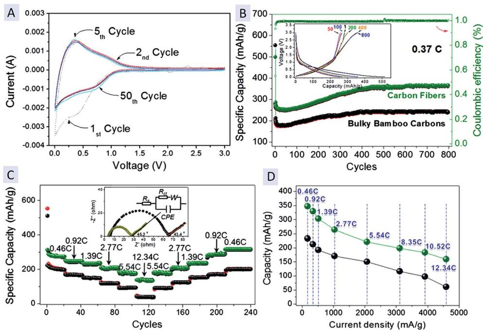
Fig. 4 (A) CV curves of carbon fibers electrode between 0.005 and 3.0 V at a scanning rate of 0.5 mV s<sup>-1</sup>. (B) Long-term cyclic performance and charge–discharge profiles, (C) programmed cyclic responses and (D) specific capacity vs. current density plot of carbon fibers (green) and bulky bamboo carbons (black). The inset in (C) shows their EIS spectra measured in a frequency range of  $1 \times 10^6$  to 0.01 Hz under open-circuit conditions.
