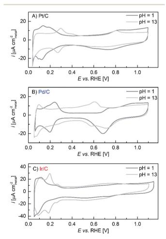
Fig. 3 Voltammograms at 293 K recorded in an Ar-saturated atmosphere at 20 mV s<sup>-1</sup> in 0.1 M NaOH (light grey line) and 0.1 M HClO<sub>4</sub> (dark grey line), except for Ir/C which was recorded in 0.05 M  $\rm H_2SO_4$  since Ir reacts with ClO<sub>4</sub><sup>-</sup> ions (see Reier *et al.*<sup>2</sup> and ref. 39–41 therein).
