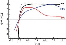
Fig. 1 Ohmic loss corrected polarization curves in a  $H_2$ -saturated atmosphere at ambient pressure and 313 K on Pt/C (black lines), Ir/C (red lines) and Pd/C (blue lines) in: (A) PEMFCs at 2 mV s<sup>-1</sup> and (B) 0.1 M NaOH at 10 mV s<sup>-1</sup> (the negative going scans are shown) and 1600 rpm. In (B), the diffusion overpotential, calculated according to Sheng et al.<sup>9</sup> is also shown (grey dashed line). For metal loadings see the ESI.†
