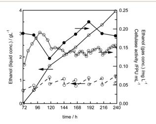
Fig. 4 Semi-continuous ethanol production from Avicel in a 16 mL MBM reactor: after a batch phase of 69 h, the Avicel concentration was adjusted to 10 g L<sup>-1</sup> and every 24 h a quarter of the reaction phase was exchanged against a fresh medium containing 10 g  $L^{-1}$  Avicel. The ethanol concentration in the liquid phase (dashed line), the ethanol concentration in the gas phase (dotted line), the cellulase activity (
