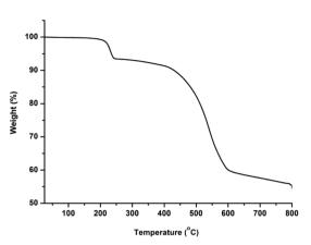
Fig. 4 Temperature dependent weight loss of CFA-5 under flowing nitrogen gas.
