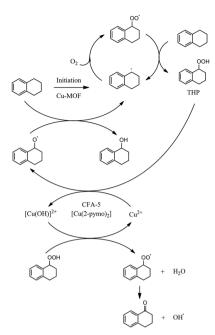
Fig. 12 Proposed reaction mechanism as a combination of homogeneous radical propagation cycles and heterogeneously catalyzed steps (initiation, THP decomposition).<sup>35</sup>
