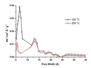
Fig. 7 Pore size distribution for CFA-5 desolvated at 100  $^{\circ}$ C (black line) and 250  $^{\circ}$ C (red line) calculated by fitting the NLDFT model to the argon sorption data.
