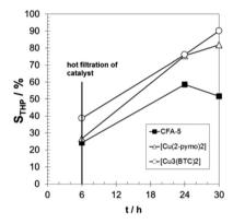
Fig. 11 Progress of THP selectivity over time with hot filtration of the catalyst after 6 h for CFA-5,  $[Cu(2-pymo)_2]$ , and  $[Cu_3(BTC)_2]$ . T = 90 °C; 20 q tetralin, tetralin/Cu molar ratio: 2000/1.
