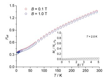
Fig. 8 Temperature dependence of the effective magnetic moment  $\mu_{\rm eff}$ per asymmetric unit of CFA-5 (cf. Fig. 3b) at 0.1 and 1.0 tesla; inset: field dependence of the molar magnetization  $M_{\rm m}$  at 2.0 K.
