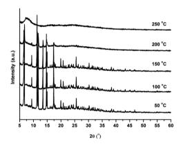
Fig. 5 VTXRPD plots of CFA-5 kept in air, sampled in a temperature range of 50-250 °C.
