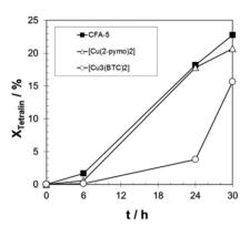
Fig. 9 Progress of tetralin conversion over time for CFA-5, [Cu(2-pymo)<sub>2</sub>], and [Cu<sub>3</sub>(BTC)<sub>2</sub>]. T = 90 °C; 20 g tetralin, tetralin/Cu molar ratio: 2000/1
