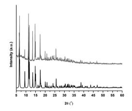
Fig. 3 Calculated and measured X-ray powder patterns for CFA-5
