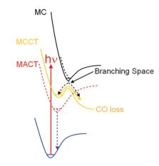
Fig. 11 A schematic representation of the low-lying excited states of  $(\eta^6$ -arene)Cr(CO)<sub>3</sub> complexes showing the lowest energy MACT excited state which is not formally optically accessible for  $(\eta^6$ -benzene)Cr(CO)<sub>3</sub> but becomes accessible for arenes containing substituents which conjugate with the arene  $\pi$ -system, and the predissociative excited state (MC) which relaxes to the spectroscopically active MCCT state.
