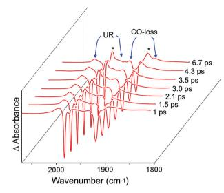
Fig. 4 Stepped offset spectra obtained following 400 nm excitation of  $(\eta^6\text{-styrene})\text{Cr}(\text{CO})_3$  in n-heptane presenting the IR spectra obtained up to 6.7 ps after excitation showing the formation of two features at 1966 and 1894 cm<sup>-1</sup> (indicated by asterisks) of an excited state precursor to CO-loss and also traces of the CO-loss species on this timescale (CO-loss).
