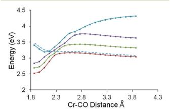
Fig. 8 The adiabatic behaviour of the four lowest energy singlet excited states for  $(\eta^6\text{-benzophenone})\text{Cr(CO)}_3$ , showing that the lowest three excited states are bound with respect to this Cr-CO reaction coordinate, while the fourth excited state (3.4 eV, 365 nm) presents an accelerating profile to CO-loss (dashed curve) in a non-adiabatic description.
