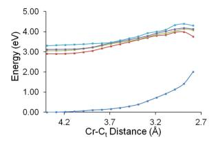
Fig. 9 The behaviour of the ground state energy and the four lowest energy singlet excited states in ( $\eta^6$ -styrene)Cr(CO)<sub>3</sub>, as the Cr–C(terminal-vinyl) distance was reduced from 4.39 to 2.79 Å in steps of 0.1 Å, showing that none of the excited states presents an accelerating profile towards a ring-slip or reduced hapticity species.
