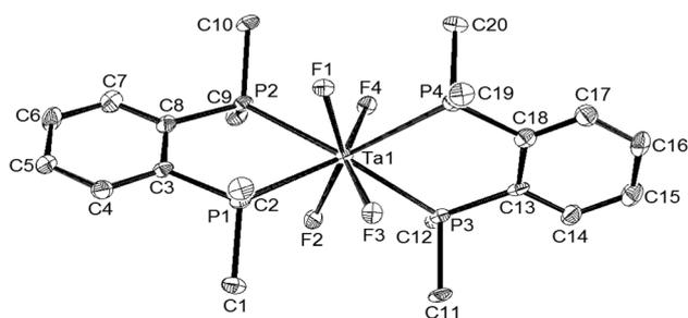
**Fig. 2** The cation of  $[\text{TaF}_4(\text{o-C}_6\text{H}_4(\text{PMe}_2)_2)_2][\text{TaF}_6]$ , ellipsoids are drawn at the 40% level. Selected bond lengths (Å) and angles ( $^\circ$ ): Ta1–F2 = 1.944(9), Ta1–F3 = 1.950(10), Ta1–F1 = 1.955(9), Ta1–F4 = 1.970(9), Ta1–P1 = 2.645(4), Ta1–P4 = 2.657(4), Ta1–P3 = 2.658(4), Ta1–P2 = 2.664(4), P1–Ta1–P2 = 71.61(13), P4–Ta1–P3 = 71.53(13), F2–Ta1–F3 = 95.5(4), F3–Ta1–F1 = 93.0(4), F2–Ta1–F4 = 92.9(4), F1–Ta1–F4 = 96.0(4).
