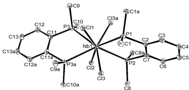
**Fig. 3** The cation of  $[\text{NbCl}_4(\text{o-C}_6\text{H}_4(\text{PMe}_2)_2)_2]\text{Cl}$ , ellipsoids are drawn at the 40% level. Selected bond lengths (Å) and angles ( $^\circ$ ): Nb1–Cl1 = 2.4309(9), Nb1–Cl3 = 2.4341(6), Nb1–Cl2 = 2.4424(10), Nb1–P3 = 2.6833(7), Nb1–P1 = 2.6843(10), Nb1–P2 = 2.6869(10), P3–Nb1–P3a = 72.32(3), P1–Nb1–P2 = 73.189(3), Cl1–Nb1–Cl3 = 94.99(2), Cl3–Nb1–Cl2 = 95.029(14). Symmetry operator a = (x, –y, z).
