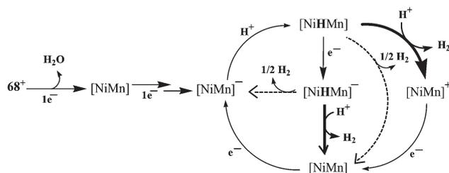
**Scheme 4** Proposed mechanisms for hydrogen evolution catalysed by [68]<sup>+</sup>. The homolytic H<sub>2</sub>-evolution steps are depicted by dotted arrows and the heterolytic steps by solid arrows (adapted from ref. 64).
