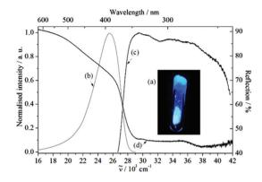
Fig. 4 (a) Violet-blue luminescence of (S)-4,4'-bis(4-carboxyphenyl)-2,2'-bis(diphenylphosphinoyl)-1,1'-binaphthyl (H<sub>2</sub>L), when illuminated with UV light. (b) Emission ( $\tilde{\nu}_{ex} = 30.864 \text{ cm}^{-1}$ ), (c) excitation ( $\tilde{\nu}_{em} = 30.864 \text{ cm}^{-1}$ ) 25 445 cm<sup>-1</sup>), and (d) reflection spectra of H<sub>2</sub>L.
