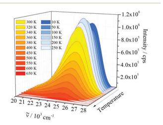
Fig. 7 Effect of temperature increase on the emission spectrum ( $\bar{\nu}_{ex}$  = 30 769 cm<sup>-1</sup>) of 1.
