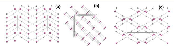
Fig. 3 Simplified two-dimensional network of 1, 3-c net, with Schläfli symbol {4.8²}, with views along the (a) [100], (b) [010] and (c) [001] direction; red spheres: Cd, grey spheres and lines: ligand representations.
