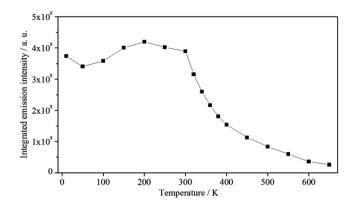
**Fig. 8** Exponential decay of the integrated emission intensity ( $\bar{\nu}_{\rm ex}$  = 30 303 cm<sup>-1</sup>) of **1** with increasing temperature.
