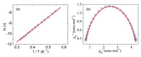
Fig. 4 (a) Arrhenius plot for 1; the solid line denotes the least-squares of maxima  $\chi_M$ " to the Arrhenius equation. (b) Cole-Cole diagram at 2.2 K for 1; the red solid line represents the least-squares fit obtained using a Debye model.
