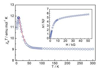
Fig. 2 Plot of  $\chi_M T$  versus T for 1 in an applied field of 1 kG from 2.0 to 300 K. The solid line represents the best fit given in the text. The inset shows a 2 K magnetization isotherm collected between 0 and 50 kG.
