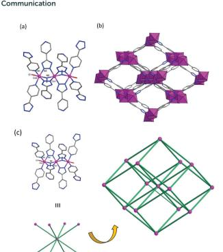
Fig. 1 (a) Local coordination environment of Co<sup>II</sup> in 1; hydrogen atoms have been omitted for clarity; (b) 3D framework of 1 constructed by a Co<sub>3</sub> subunit (shown in polyhedron); (c) simplified view of an eightconnected Co<sub>3</sub>L<sub>8</sub> node and perspective view of the network of 1 to the bcu net topology.
