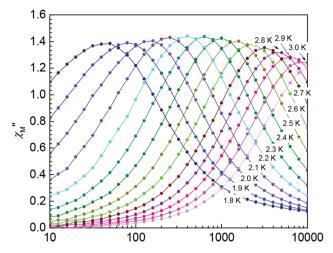
Fig. 3 Plots of out-of-phase ( $\chi_M$ ") of AC susceptibility vs. frequency in a 3.5 G AC field oscillating and 500 G DC field at the indicated temperatures for complex 1.
