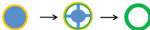
Fig. 9 Hollowing by the Kirkendall effect.
