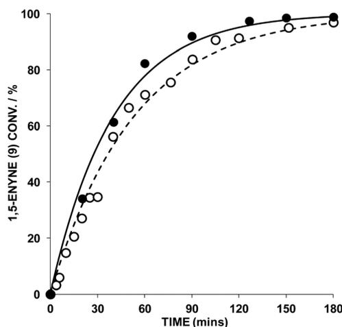
Fig. 2 Effect of AgOTf equivalents relative to AuBr<sub>2</sub>(*N*-TFS)(*I*<sup>t</sup>Pe) in 1,5-enyne cycloisomerisation of 9 (key: ● = 2 mol% AgOTf; ○ = 1 mol% AgOTf). Other details: [9] = 0.2 M, DCE, 1 mol% Au cat., 25 °C; 1,5-enyne conversion was monitored by HRGC – each sample point was quenched by addition of *N*(*n*-Bu)<sub>4</sub>Br. The kinetic curves were fitted using Dynafit™.
