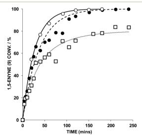
Fig. 4 Effect of 1,5-enyne concentration [9] in a reaction mediated by  $AuBr_2(N-phthal)(I^tPe)$  (1 mol%), AgOTf (1 mol%), in DCE at 25 °C (key:  $\circ$  = 0.1 M 9;  $\bullet$  = 0.2 M 9;  $\Box$  = 0.5 M 9). 1,5-Enyne conversion monitored by GC analysis - each sample point was guenched by addition of (n-Bu)<sub>4</sub>NBr. The kinetic curves were fitted using Dynafit<sup>TM</sup>.
