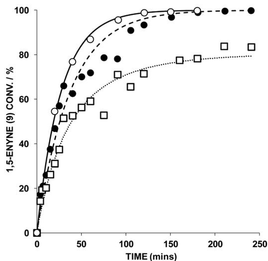
Fig. 4 Effect of 1,5-enyne concentration [**9**] in a reaction mediated by AuBr<sub>2</sub>(N-phthal)(I<sup>t</sup>Pe) (1 mol%), AgOTf (1 mol%), in DCE at 25 °C (key: ○ = 0.1 M **9**; ● = 0.2 M **9**; □ = 0.5 M **9**). 1,5-Enyne conversion monitored by GC analysis – each sample point was quenched by addition of (*n*-Bu)<sub>4</sub>NBr. The kinetic curves were fitted using Dynafit™.
