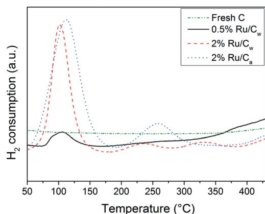
Fig. 4 H<sub>2</sub>-TPR profiles of the fresh C, 0.5% Ru/C<sub>w</sub>, 2% Ru/C<sub>w</sub>, and 2% Ru/C<sub>a</sub> catalysts.
