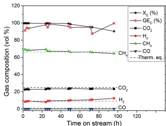
Fig. 7 CSCWG of 10 wt% isopropanol over the 2% Ru/C<sub>a</sub> catalyst at 450 °C and 30 MPa for 96 h on-stream with  $WHSV_{gRu} = 1228 \text{ g}_{Org} \text{ g}_{Ru}^{-1} \text{ h}^{-1}$ . The dashed lines denote the calculated thermodynamic equilibrium concentrations.
