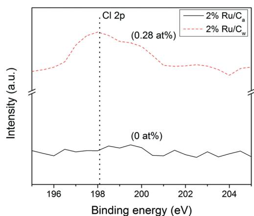
Fig. 3 Cl 2p (198.1 eV) XPS patterns of 2% Ru/C<sub>w</sub> and 2% Ru/C<sub>a</sub> catalysts.
