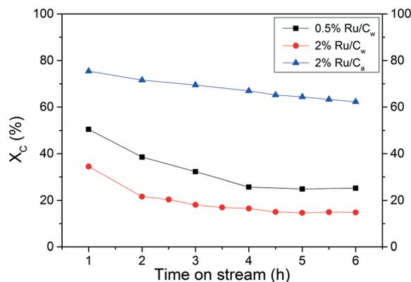
Fig. 8 Assessment of the Ru dispersion effect and the solvent effect during CSCWG of 10 wt% isopropanol at 450 °C and 30 MPa with  $WHSV_{gRu} = 5202 \text{ g}_{Org} \text{ g}_{Ru}^{-1} \text{ h}^{-1}$ .
