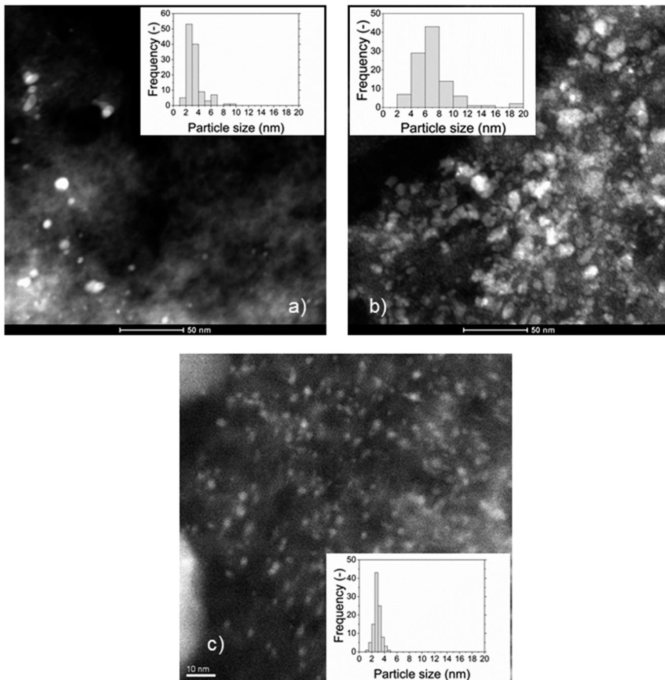
**Fig. 2** HAADF-STEM images of the (a) 0.5% Ru/C<sub>w</sub>, (b) 2% Ru/C<sub>w</sub>, and (c) 2% Ru/C<sub>a</sub> catalysts.
