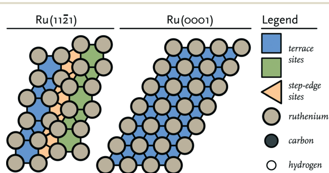
Fig. 1 Schematic representation of (left) the corrugated Ru(11 \bar{2} 1) surface and (right) the close-packed Ru(0001) terrace surface.
