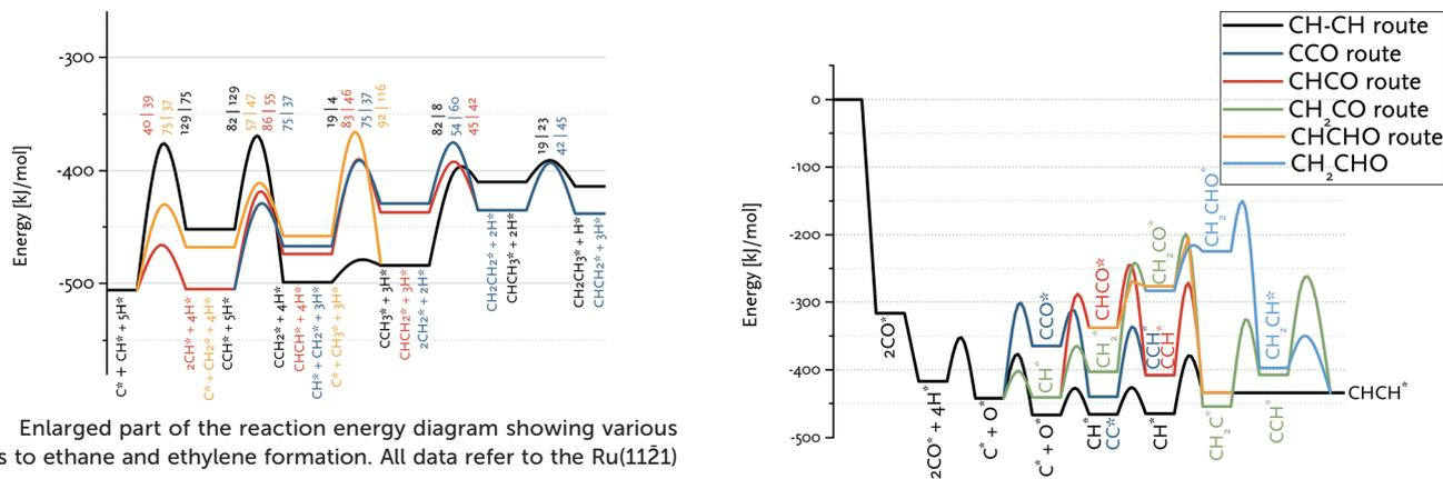
Fig. 7 Enlarged part of the reaction energy diagram showing various routes to ethane and ethylene formation. All data refer to the Ru(1121) surface.
