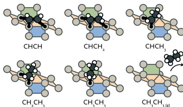
**Fig. 3** Schematic representation of hydrogenation of adsorbed acetylene to ethane.
