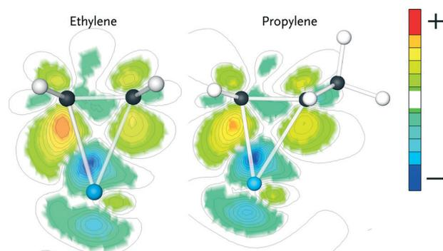
**Fig. 5** Electron density difference plots of the adsorbed states of ethylene (left) and propylene (right) on the Ru(1121) surface. These plots were generated by subtracting the electron density of the individual complexes in vacuum and empty surface from the electron density of the complex. Note that the electron density difference for ethylene is larger than for propylene.
