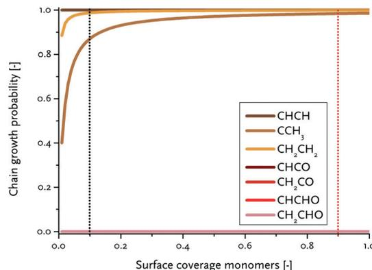
**Fig. 10** Computed chain-growth probability ( $\alpha$ ) as a function of the surface coverage of the chain propagating surface intermediate (CH in the carbide mechanism and CO in the CO insertion mechanism). The black and red dotted lines indicate typical respective  $\text{C}_1$  and CO coverage encountered under typical FT reaction conditions.
