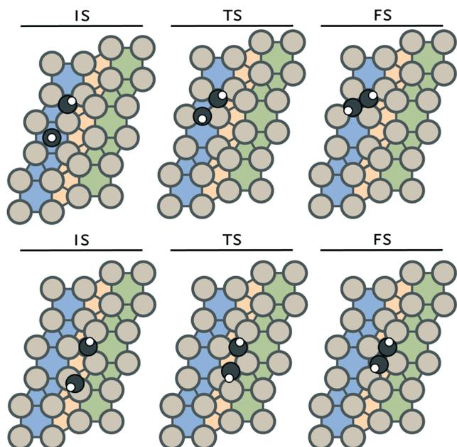
**Fig. 2** Schematic representation of the two CH + CH coupling pathways on the Ru(11 $\bar{2}$ 1) surface. The coupling of two CH moieties on (top) a terrace site and (bottom) a step-edge site. The black and white spheres represent carbon and hydrogen atoms, respectively.
