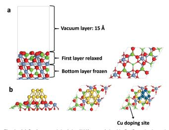
Fig. 1 (a) Surface model of the (111)-cut of the MgCr<sub>2</sub>O<sub>4</sub> spinel used; (b) Au cluster (left: top view; middle: side-on view) consisting of a Au<sub>10</sub> cluster adsorbed on the (111)-cut of the MgCr<sub>2</sub>O<sub>4</sub> spinel structure (one out of four Mg cations in the surface indicated by the arrow is replaced by a Cu substituent; color scheme - red: O; yellow: Au; green: Mg; blue: Cr; orange: Cu).
