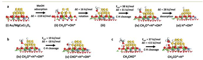
Fig. 5 (a) Mechanism of oxidation of methanol to formaldehyde for the Au<sub>10</sub>/MgCuCr<sub>2</sub>O<sub>4</sub> model. From state v, the recombinative desorption of water is similar to the mechanism found for ethanol oxidation (states v-ix in Fig. 2); (b)  $\alpha$ -C-H bond cleavage in adsorbed formaldehyde and (c)  $\alpha$ -C-H bond cleavage in adsorbed acetaldehyde.
