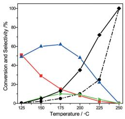
Fig. 6 Conversion and selectivity of methanol oxidation (0.1 g of catalyst, 5 vol% methanol, methanol/O2/He ratio = 1/3/16, GHSV = 60 000 mL  $g_{cat}^{-1}$   $h^{-1}$ ) as a function of the reaction temperature (ullet: methanol,  $\blacksquare$ : formaldehyde,  $\underline{\wedge}$ : methyl formate,  $\underline{\triangleright}$ : formic acid, ♦: carbon dioxide).
