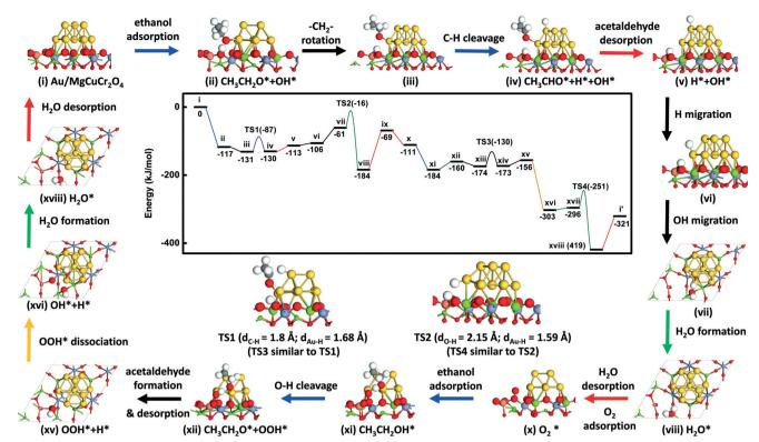
Fig. 2 Mechanism of oxidation of ethanol to acetaldehyde for the Au<sub>10</sub>/MgCuCr<sub>2</sub>O<sub>4</sub> model: (center top) reaction energy diagram, (center bottom) most important transition state structures and (periphery) reaction mechanism (DFT calculations for the Au<sub>10</sub> cluster on the (111) surface of MgCuCr<sub>2</sub>O<sub>4</sub>; cut-off energy set at 400 eV).
