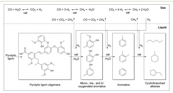
Fig. 8 The proposed global network for the catalytic hydrotreatment of pyrolytic lignin with Ru/C.
