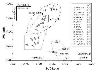
Fig. 3 The van Krevelen plot for the feeds and products of the catalytic hydrotreatment reaction (400 °C, 100 bar H<sub>2</sub> initial pressure, 4 h. 5 wt% of Ru/C) and literature data for PL
