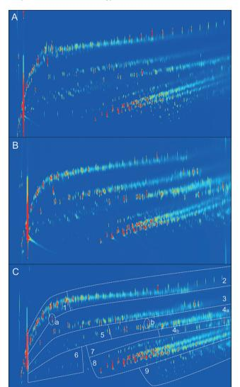
Fig. 5 GCxGC-FID chromatograms of the organic phase from A) Alcell LO, B) pine PLO, and C) forestry residue PLO. 1 = mainly cyclic alkanes, 2 = mainly linear/branched alkanes, 3 + 4 = aromatics, 4a = napthalenes, 4b= polycyclic aromatic hydrocarbons, 5 = ketones/ alcohols, 6 = acids, 7 = guaiacols, 8= alkylphenolics, 9 = catechols. Also a = internal standard and b = BHT (stabilizer in THF).
