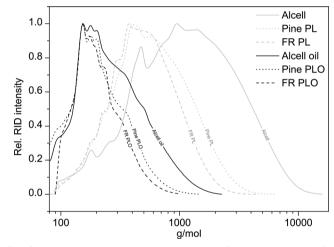
Fig. 6 Molecular weight distribution of pine PL, forestry residue PL, organosolv Alcell lignin, and the corresponding hydrotreated lignin oils (400 °C, 4 h, 100 bar initial H<sub>2</sub>, 5 wt% Ru/C).
