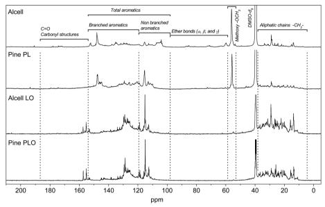
Fig. 7 13C-NMR spectra of two feeds (Alcell and PL from pine) and their product oils after catalytic hydrotreatment.
